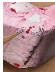
Visible Penetrant Indications
