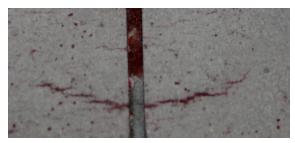
High temperature penetrant VP-302 crack indication on D-702 developer film.
