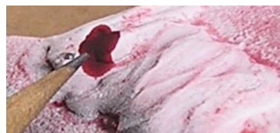
Visible Penetrant Indication on Weld
