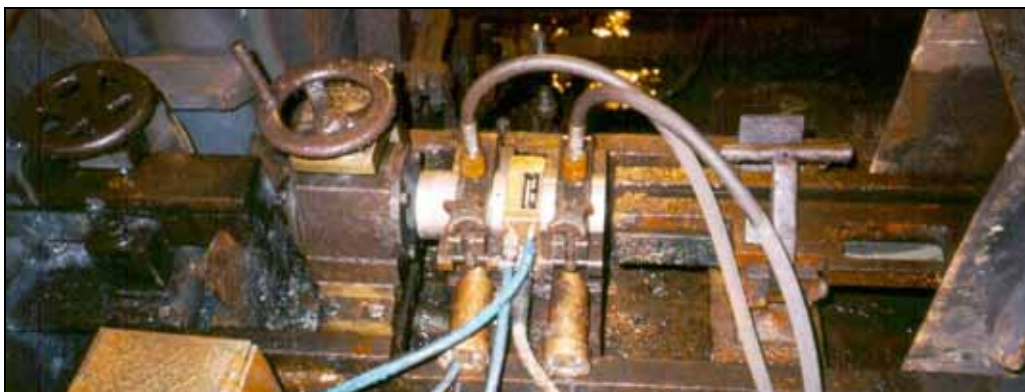
Figure 1: Sensor system T 60, installed in a hot wire line
