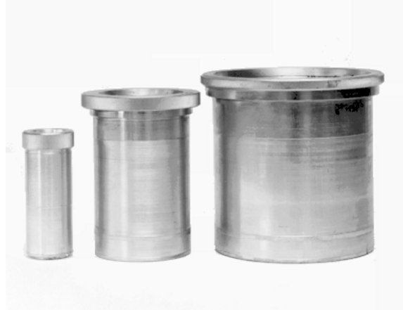
Figure 7: Protective nozzles for different test piece diameters
