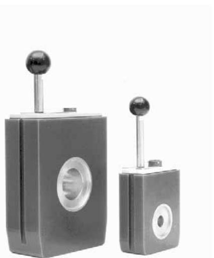
Fig. 4 LMD test coils of various diameters
