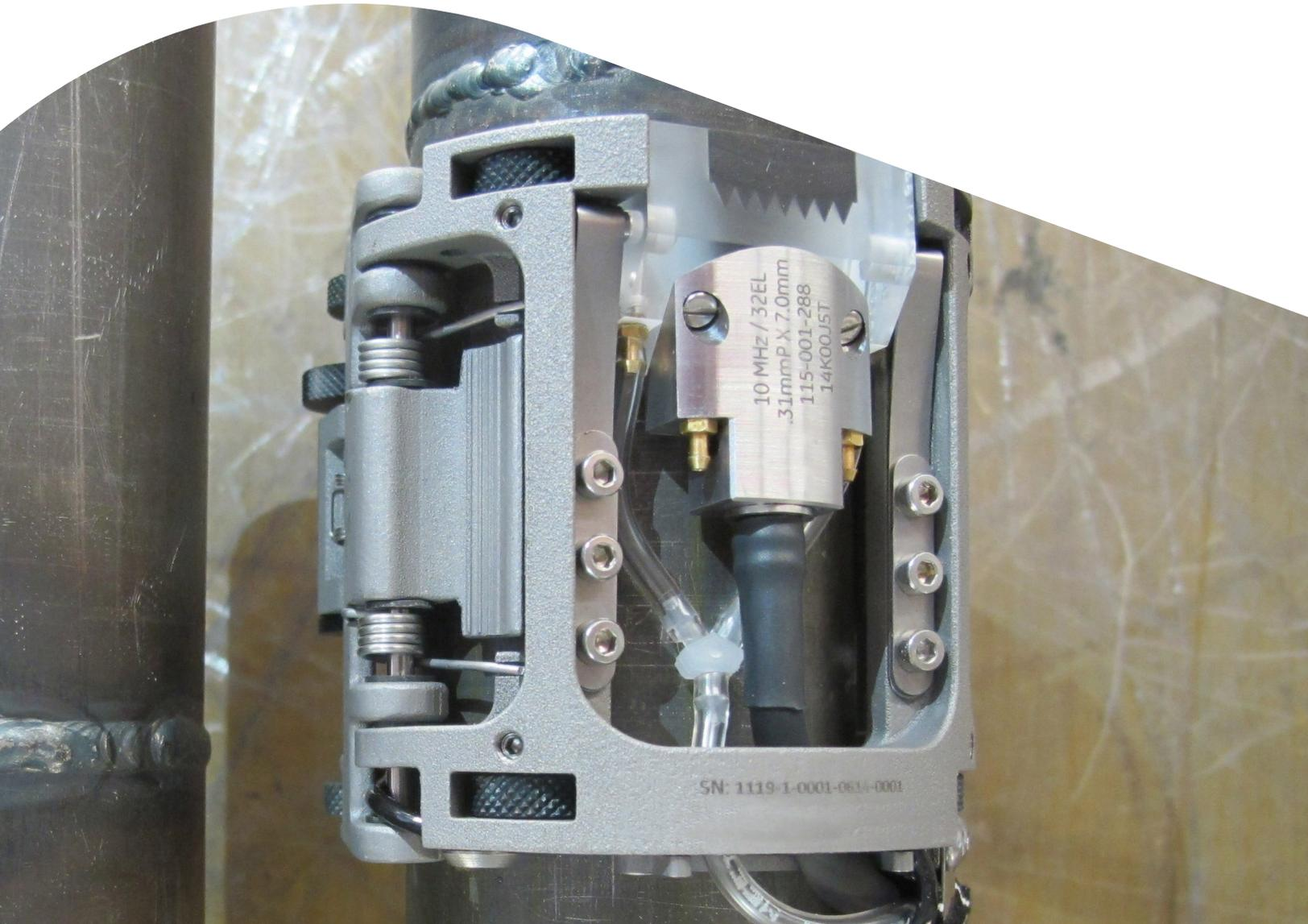
NDT inspections of circumferential butt welds are a complex task. This type of joint is found in various structures including small diameter tubes in boilers. Experts inspect these to find defects which could result in the failure of a component, possibly inducing a human or environmental hazard.
