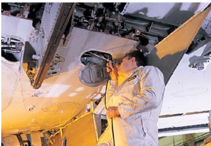
Inspection of hard-to-reach area of airframe structure
