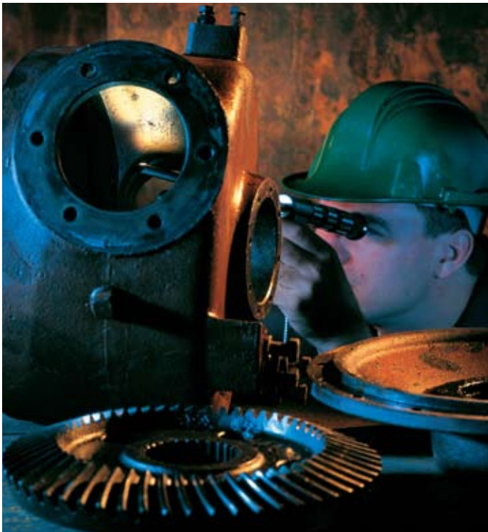
Rigid Borescope inspection of power take-off transmission
