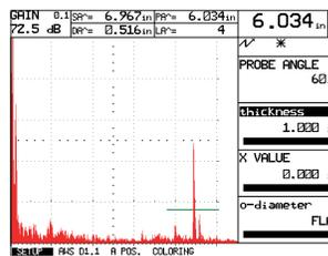
Four digital reading boxes at top display trigonometric calculations for weld inspection.
