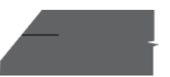
51 Lamination in Weld Prep MT/PT, UT
