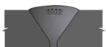
30 Porosity in Single Vee (sub-surface) UT, RT
