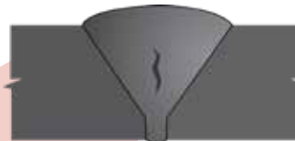
15 Centerline Crack, Single Vee (sub-surface) UT, RT
