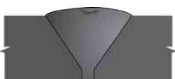
20 Crater Crack (crown stop-start area) MT/PT, UT
