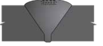
32 Porosity in Single Vee (surface breaking) VT, MT/PT
