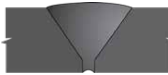
70 Root Concavity in Single Vee VT, RT
