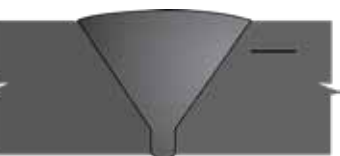
50 Lamination in Single Vee (base metal) UT
