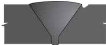
78 Undercut in Single Vee, VT
