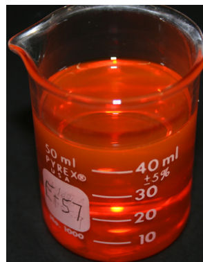
Fluorescent Penetrant Indications Type 1, Method B, Level 2, form "a"
