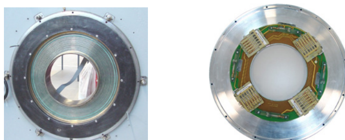
Fig. 13: Disc slip ring (left) and flange with brush blocks (right)
