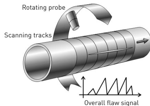
Fig. 3: Scanning tracks and defect signal
