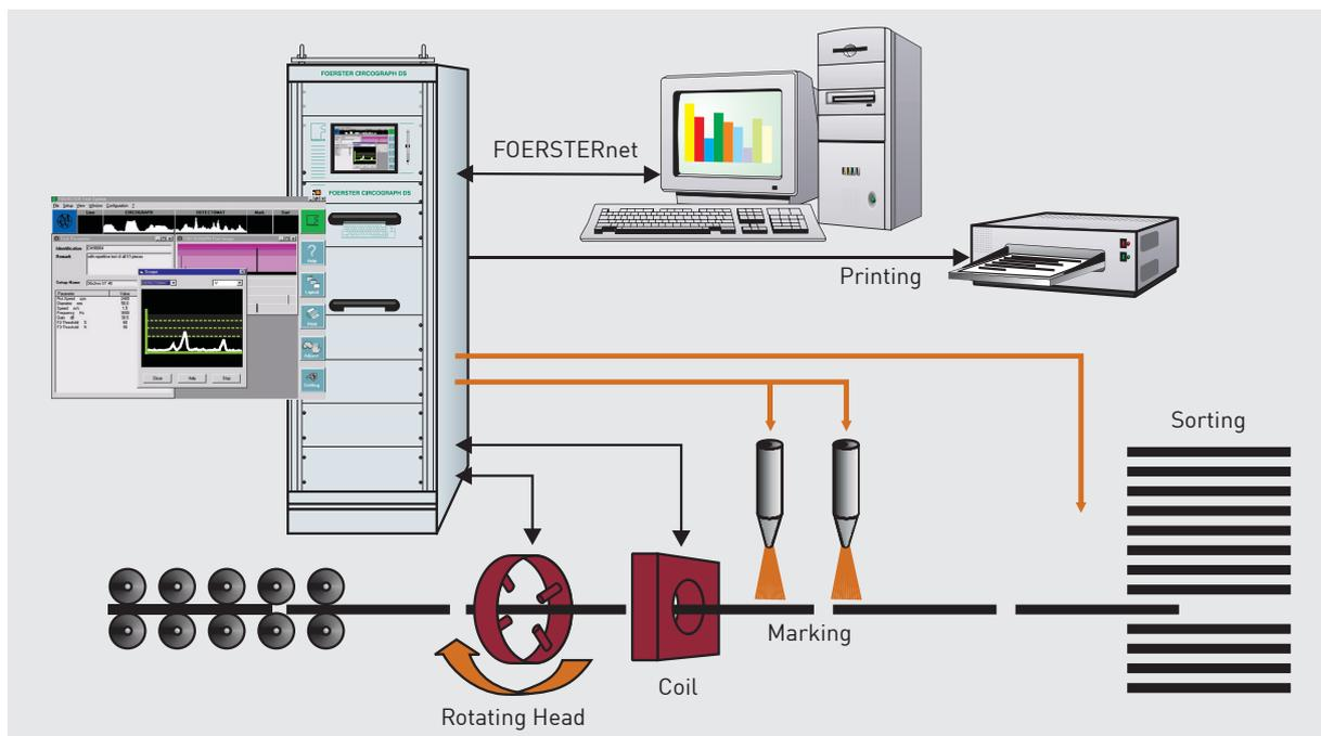
Fig. 1: Application CIRCOGRAPH with DEFECTOMAT channel for piece testing
