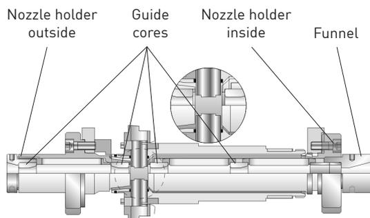
Fig. 18: Principle of precision guide using guide cores
