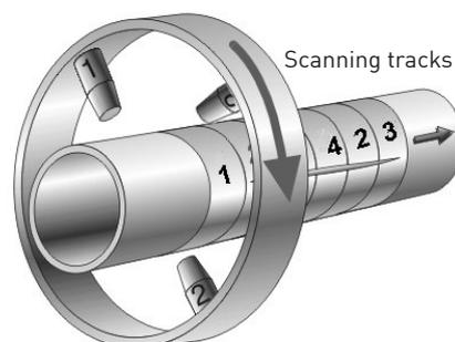
Abb. 4: Scanning tracks with four probes (90° offset)
