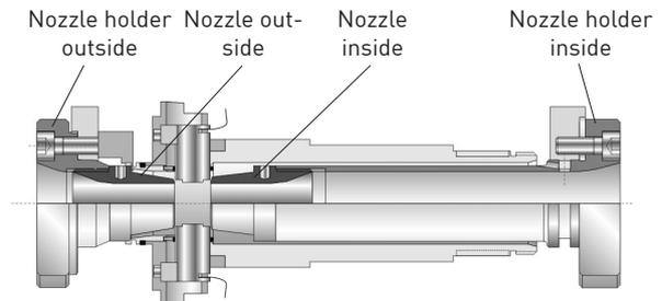
Fig. 16: Principle of protective nozzles and nozzle holder standard
