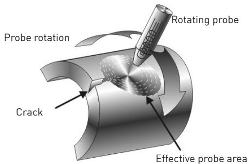
Fig. 2: Rotating probe at material defect
