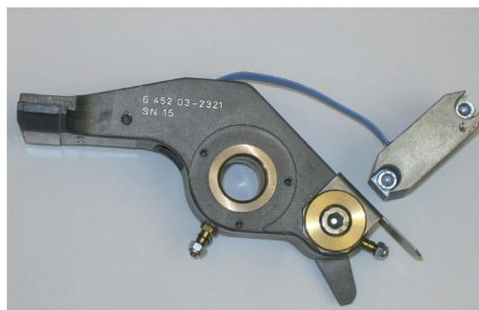
*Fig. 9: Test head in lever design*
