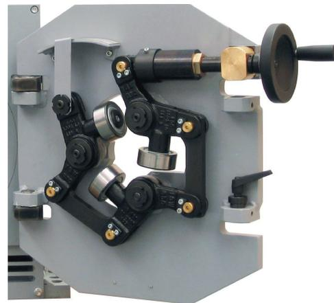
Fig 14: Triple roller guide
