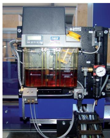
Fig. 19: Oil Air Lubrication
