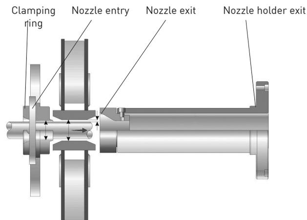
Fig. 17: Principle of protective nozzles and nozzle holder robust
