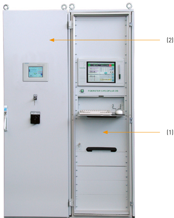
Fig. 2: CIRCOFLUX testing and evaluation electronics
